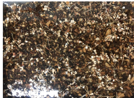
Fig 5: Soaked coconut shell aggregate
