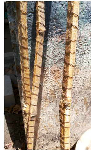
Figure 4: Treated bamboo with binding wire
